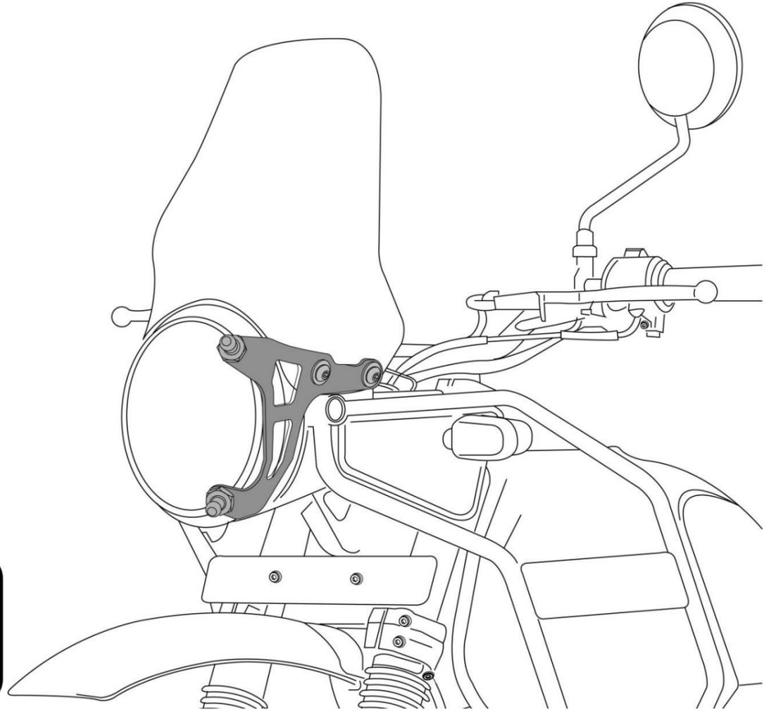
**Bracket RH (5) in “As Is Mounted Condition”**
