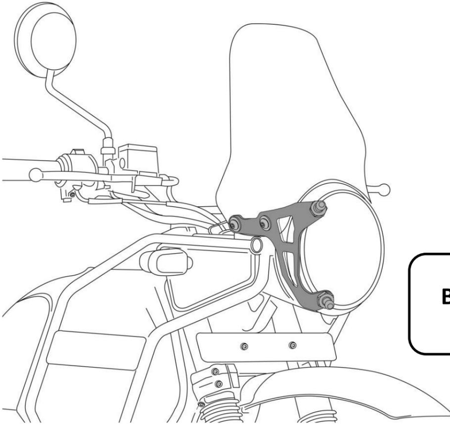
**Bracket RH (2) in “As Is Mounted Condition”**
