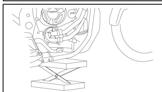
Before starting to mount, we have to Use the jack to lift the motorbike (as shown)
